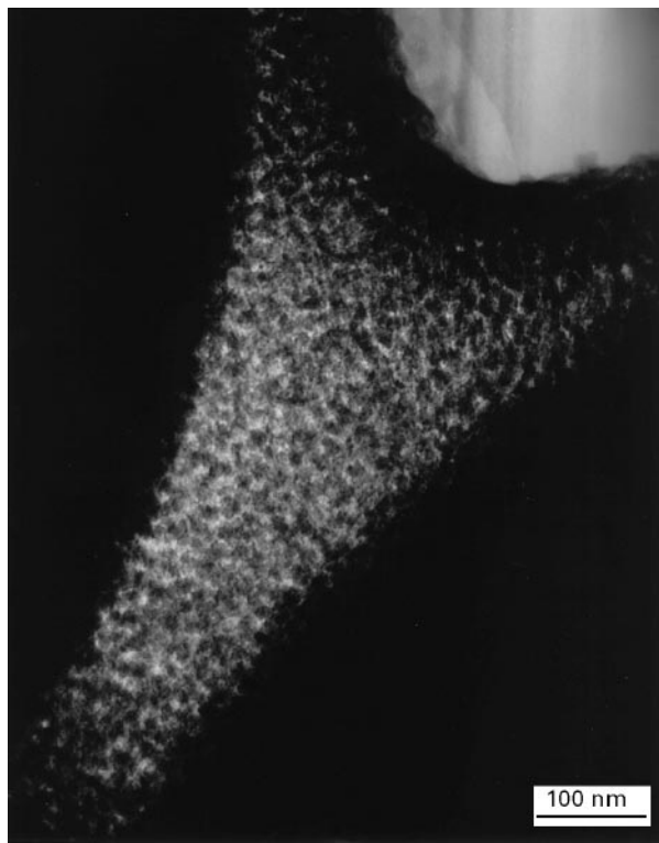
Figure 1 Bright-field TEM image of MMC sample A showing portions of two Fiberfrax® fibres joined by a porous web of silica sol particles from the silica binder used in the fibre preform. A section of the aluminium alloy matrix appears in the upper right corner. In this sample, the fibre preform was calcined at 850 °C prior to melt infiltration and the MMC was T5 treated.
